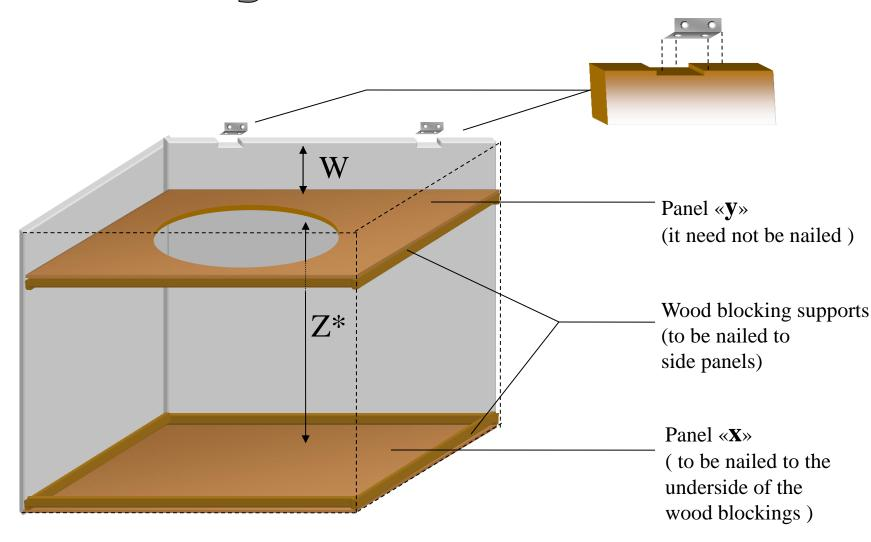
W is a recess to house the receptacle's handle. W must be as small as possible! (W depends on your type of receptacle).  $Z^*$  depends on the receptacle height. If the receptacle is smaller, panel «X» will be adjusted accordingly (positioned higher with respect to the lower edge of the side panels).
